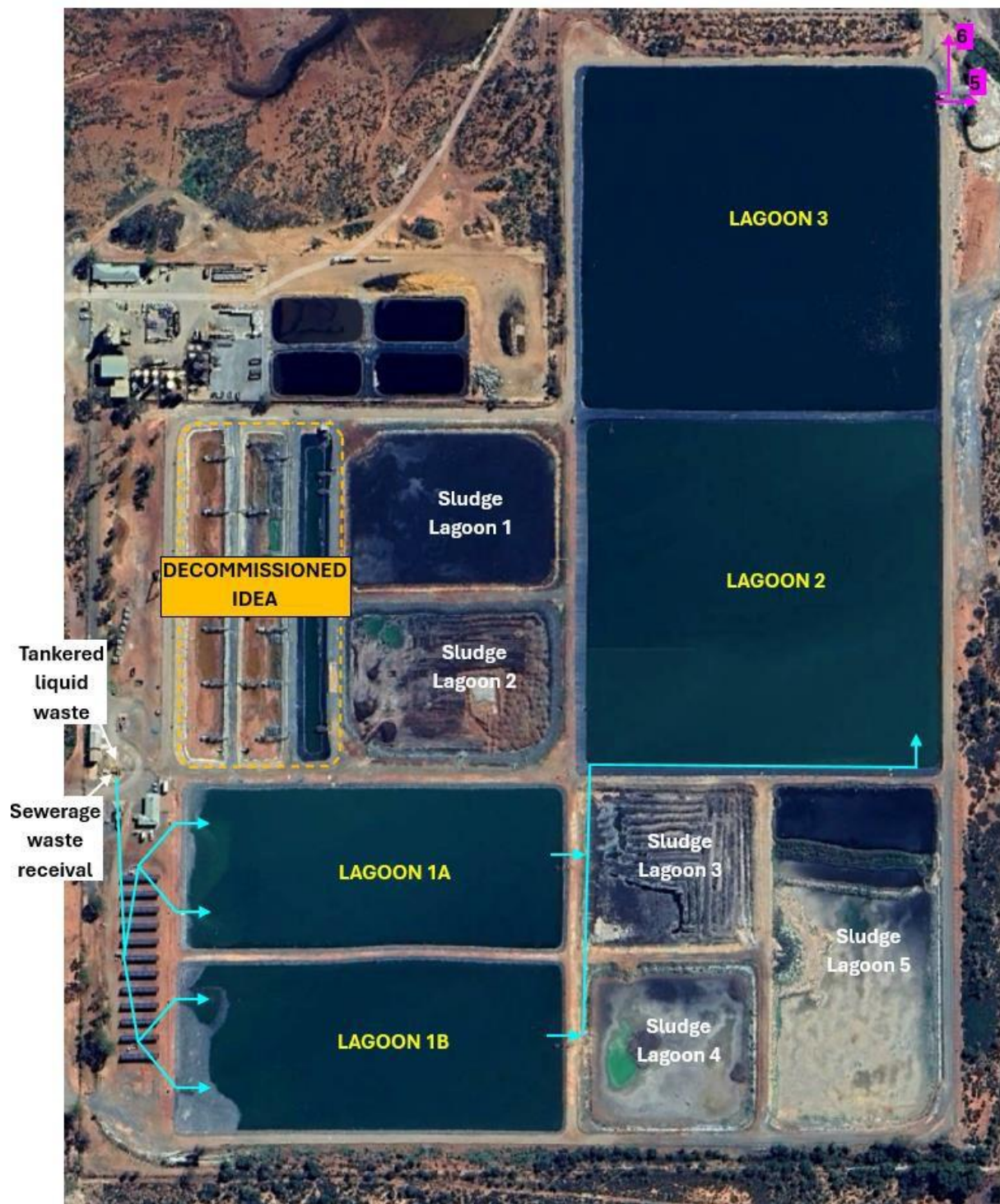
Figure 4: Current configuration of the SBWWTP
